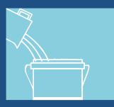
Add 400ml of GRESBOND Premium Grout Admix KGA-01 in 1 kg grout and mix until a slump free & smooth grout is obtained.
