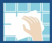
Apply mixture to the surface and work it well into the joints ensuring that they are completely filled.
