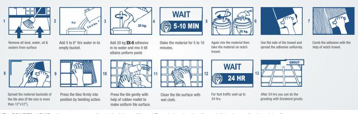
\* The POWDER: LIQUID ratio may vary according to the job conditions \*\*For exterior elevation tiles, add latex base adhesive mixture"
