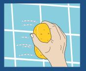
Remove excess grout while working diagonally over the area to be grouted.
